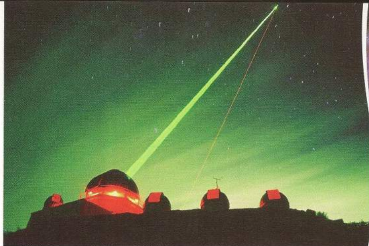
▲ Lasers beam from telescopes at the Starfire Optical Range in New Mexico. Such adaptive optics (AO) systems allow astronomers to create clearer images of stars.
