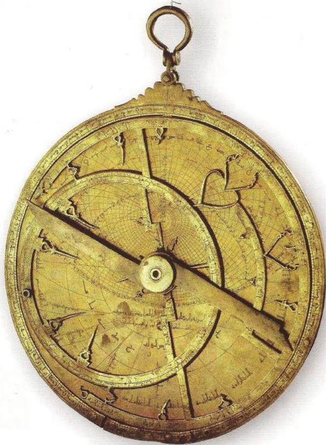
▲ This astrolabe was used by the Moors to locate and predict the positions of the sun, moon, planets, and stars. It thus served as a tool for navigation, surveying, and timekeeping.
