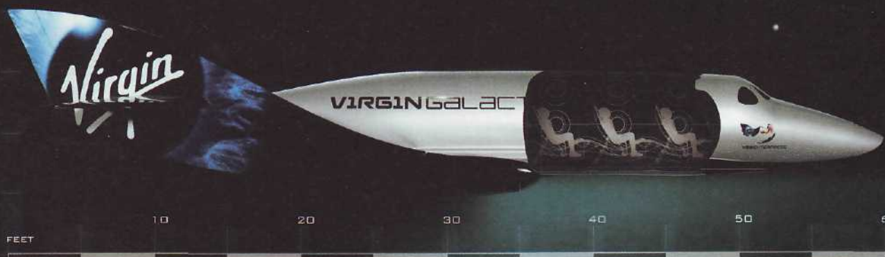
▲ Virgin Galactic's SpaceShipTwo , at 18 meters long (60 feet), will be twice as long as the original SpaceShipOne . It will carry six passengers and two pilots aboard.
