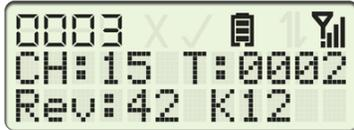
For example, this summary screen shows that pad ID 3 (0003) is programmed to communicate on channel number 15 (CH:15). Notice that the lower right of the screen must show K12 (not HE) to work with ExamView.
